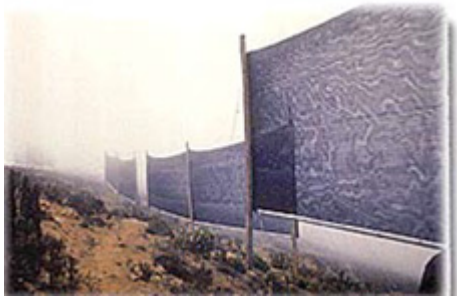
Fog collectors in El Tofo, Chile. Ph.Journaldunet
